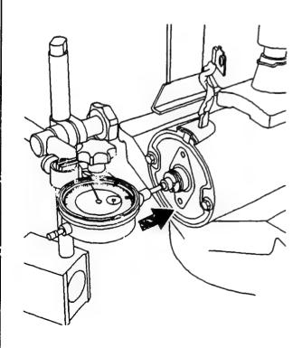
Checking and adjusting armature axial clearance
